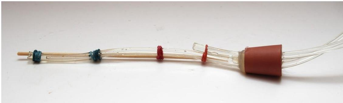
2) Pour water into the plastic bottle, so it is almost full and close the bottle with the rubber plug with tubes. Connect the tubes to the sensor, which was placed above. See the USB link to connect the sensor to the notebook. Pay attention to water, so it does not wet the sensor.
