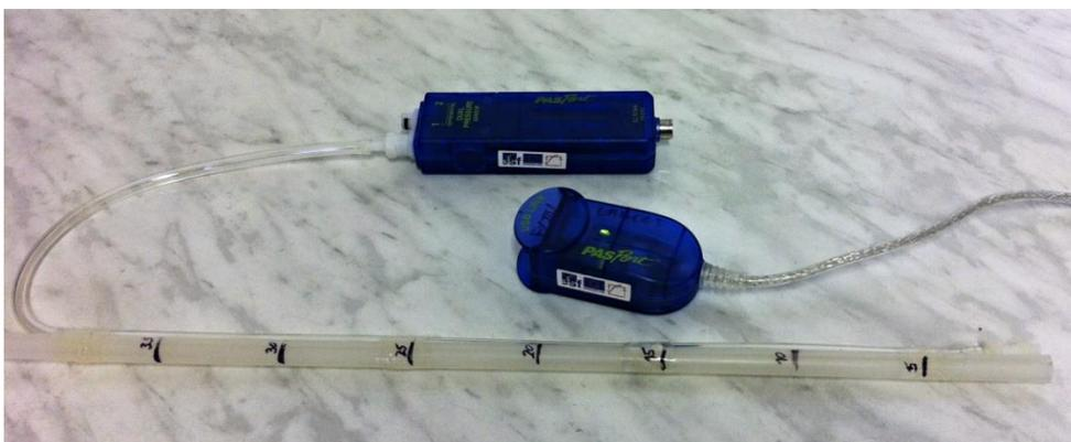
2) Pour water into the aquarium, connect the pressure sensor to the USB link and to the notebook.
