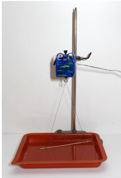
3) Set the sampling frequency to 10Hz in Setup in the DataStudio program. Set the visualising of the graph of force – time relationship.
